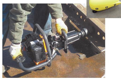
The I" Gas Impact Wrench is designed to tighten and loosen track bolts and lag screws.
